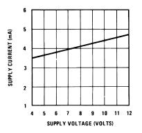
Figure 11. Supply Current vs Supply Voltage
