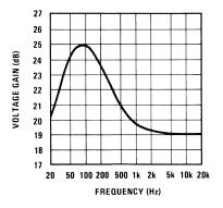
Figure 19. Voltage Gain vs Frequency
