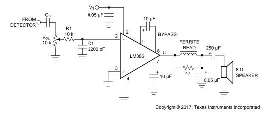
Figure 22. AM Radio Power Amplifier
