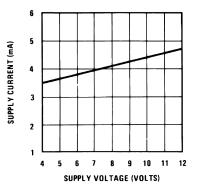
Figure 15. Supply Current vs Supply Voltage
