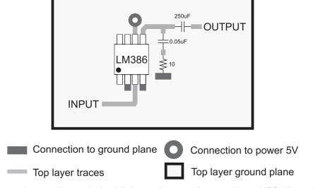
Figure 26. Layout Example for Minimum Parts Gain = 20 dB on VSSOP package
