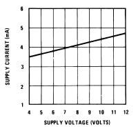
Figure 21. Supply Current vs Supply Voltage
