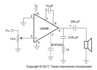
Figure 12. LM386 with Gain = 200
