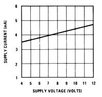
Figure 13. Supply Current vs Supply Voltage
