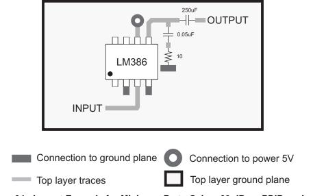
Figure 24. Layout Example for Minimum Parts Gain = 20 dB on PDIP package
