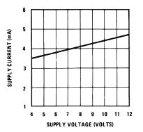
Figure 23. Supply Current vs Supply Voltage
